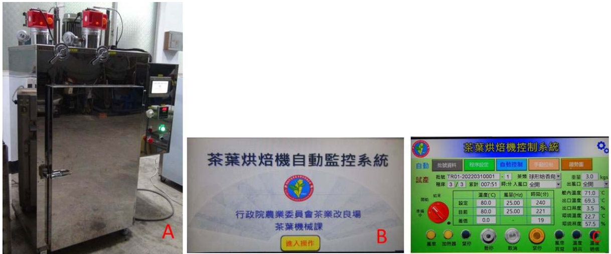
圖一、具有監控系統之茶葉烘焙機 A：茶葉烘焙機；B：人機介面；C：操作畫面 Fig. 1. Tea roasting machine with monitoring system A: tea roasting machine B: human machine interface C: operation screen
