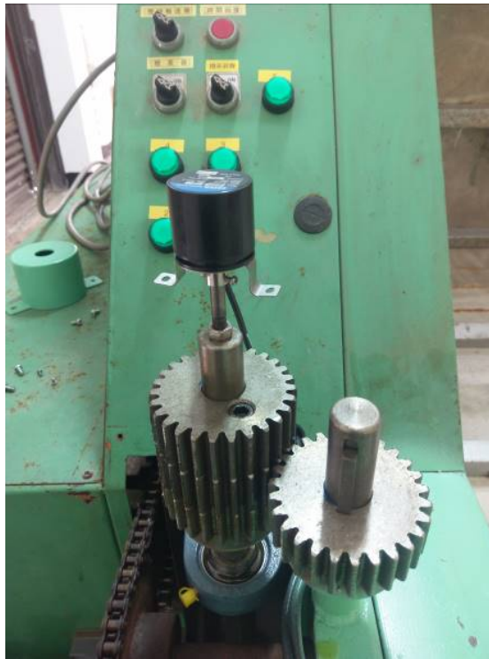
圖二、裝設電磁式轉速譯碼器監控茶菁撥桿之高度 Fig. 2. Installation of a magnetic rotary encoder to monitor the height of the rotary tea rake
