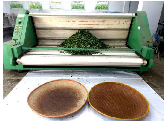
圖三、茶菁 25 公斤可直接倒入攪拌機內 Fig. 3. 25 kg of tea leaves can be poured directly into the stirring machine
