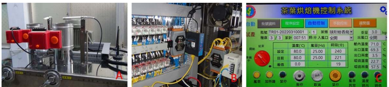
圖二、烘焙機監控系統 A：溫溼度感測器；B：訊號轉換器與通訊模組；C：遠端監控畫面 Fig. 2. The monitoring system of tea roasting machine A: temperature and humidity sensor B: signal converters and communication modules C: remote monitoring screen
