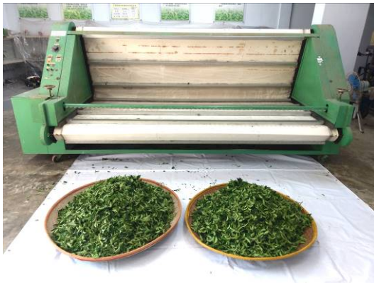
圖三、茶菁 25 公斤可直接倒入攪拌機內 Fig. 3. 25 kg of tea leaves can be poured directly into the stirring machine
