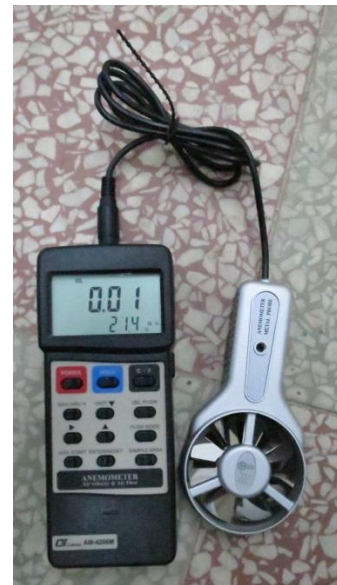
圖九、風量計 (型號：AM-4206M) Fig. 9. Air flow meter (model: AM-4206M)
