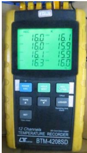
圖五、溫度記錄器 (型號：BTM-4208SD) Fig. 5. Temperature recorder (model: BTM-4208SD)
